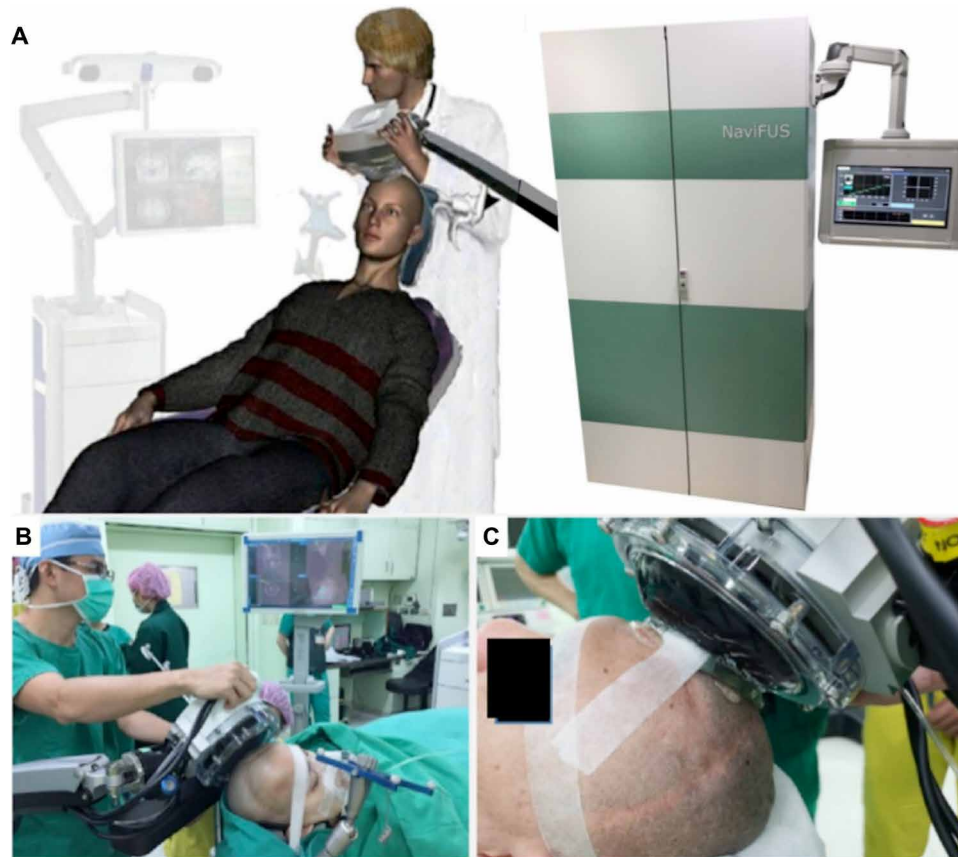
Fig. 7. Schematic diagram of neuronavigation-guided FUS treatment. (A) The system is constructed by a FUS phased array system in conjunction with neuronavigation system to intraoperatively guide FUS energy deposition in targeted brain regions. A patient is fixed semirigidly without headpin system. (B and C) The phased array probe is connected to the power generator and working station by a mechanical arm, which can be adjusted by a physician to match the trajectory and target according to the guidance of neuronavigation. The whole procedure takes less than 1 hour. Photo credits: Ko-Ting Chen, Chang Gung Memorial Hospital at Linkou, Taoyuan, Taiwan.
